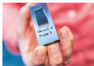
Material fatigue: A steel sample after the abrasion test.
